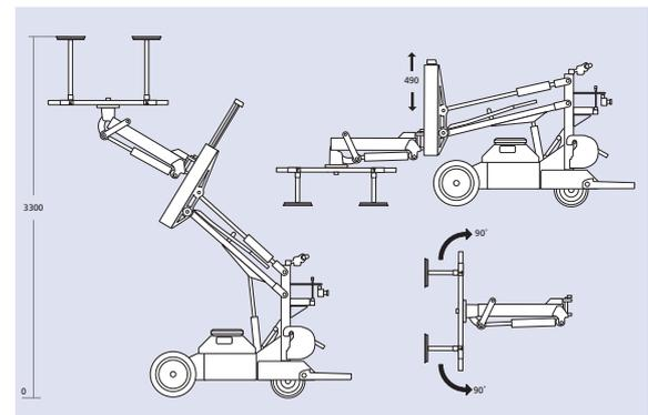
With the horizontal lifting arm as an optional extra you are able to pick up loads from ground level and mount it up to 3,2 meters.
