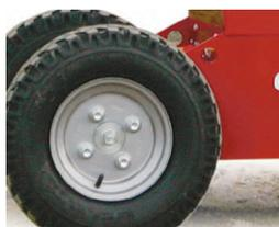
The Glaslift® has a differential front wheel drive and rugged rubber tires, this means superior traction, precision and agility. Furthermore traction will increase proportionally with the load weight.
