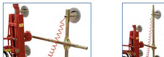
The construction of the extension bar enables it to extend the horizontal main frame as well as the vertical cross bar on the standard machine.
