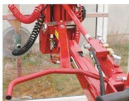
2 x 50 mm sideshift allows the operator to manipulate loads millimeter precise sideways. This is a great feature for granite slabs, plasterboard and glass fitting jobs.
