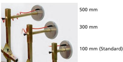
Extension arms for suction discs allows you to extend the fitting area forwards. 100 mm arms are standard on delivery. Extension arms are available as extras in 300 mm and 500 mm.
