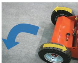
Allows the Glaslift® to turn "on the spot". The turning radius is not more than its own length, because the differential adjust the rotation of the front wheels automatically.
