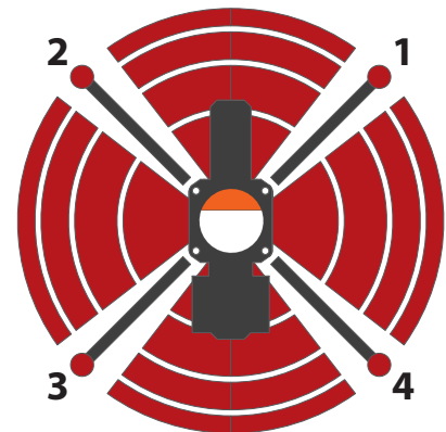
If even a single outriggers is not on the ground no possible movement is permitted.
